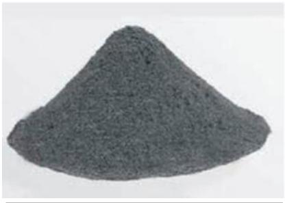
High purity atomized Al (88.5 vol. %)
