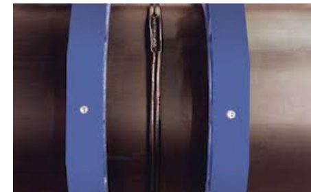
Fusion Bonded HDPE Joint
