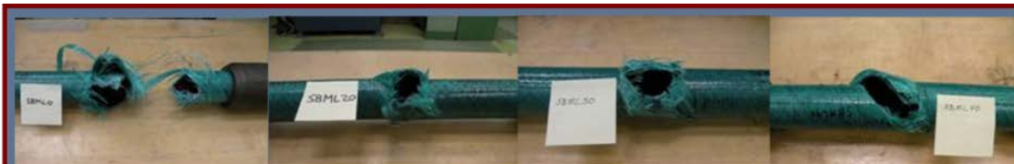
Failure mode changes from global to local and then move back towards global as flaw depth increases
